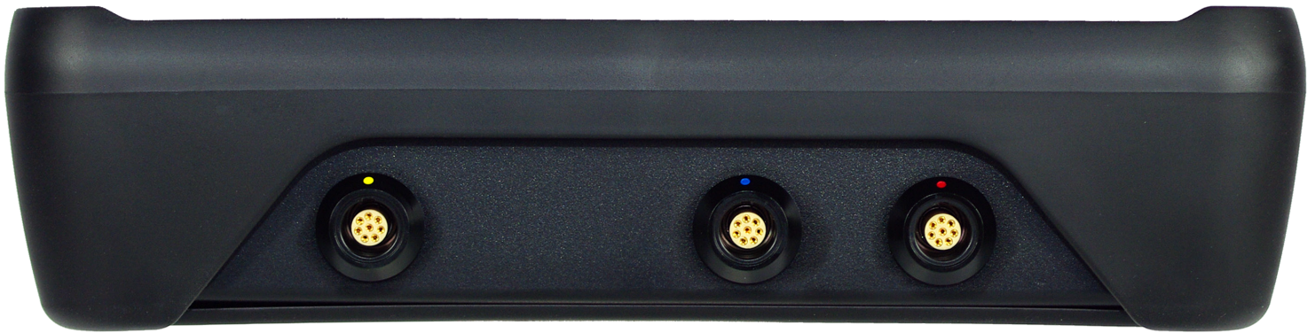
Front view containing vibration inputs for left and right plane and the tachometer sensor
